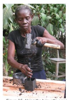
Figure 16: Using the briquette press Photo credit: Fuel from the Fields.
