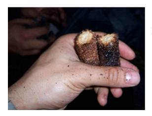
Figure 15: Corn cobs that are not completely carbonised. Photo credit: Fuel from the Fields.
