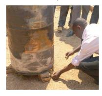
Figure 9: Raise the drum on three flat stones, and light the wicks at the bottom. Photo credit: Fuel from the
