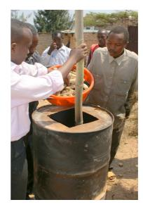
Figure 7: Fill the drum with a central chimney. Photo credit: Fuel from the Fields.
